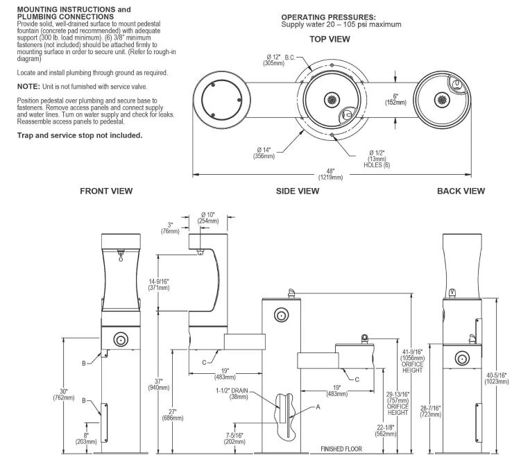
A = 3/8" O.D. Unplated copper tube connect. Shut off valve by others.
